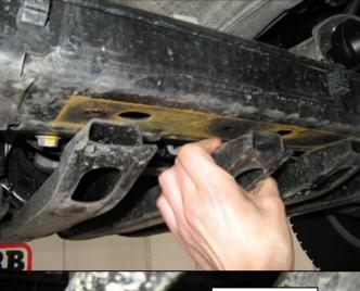
Remove rear mounting bolts from front skid rails. Pull away from chassis slightly. This must be done to gain clearance to fit front bracket.
