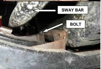
3. Slide front mounting assembly onto front cross member from left hand side of vehicle. Place an M8 cage nut onto cage nut plate and feed through access hole on bottom of cross member (bend to shape). Secure loosely using M8 x 25 bolt, spring washer and flat washer.
