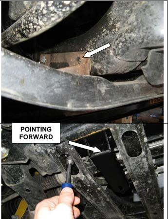
5. Once bracket is in correct position mark other hole using a white marker pen. Remove bracket and drill hole using 9mm drill bit. Refit bracket when done and secure with an extra cage nut plate, M8 cage nut, M8 x 25 bolt, spring washer and flat washer. Adjust bracket once again as per step 4.
