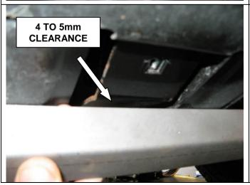
4. Make sure there is 4 to 5mm clearance between bottom edge of skid rails and folded lip of front bracket.
