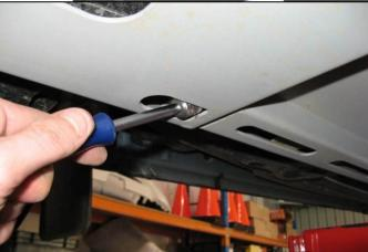
11. Lift transmission panel into place and secure front using 3 x M8 x 25 bolts, spring washers and flat washers. Leave finger tight.
