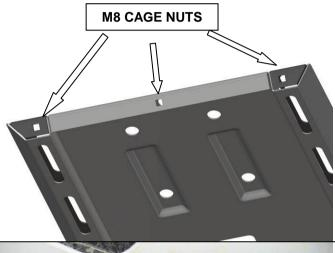
10. Fit 3 x M8 cage nuts to inner surface of transmission panel.
