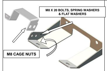
Bolt the two front brackets together as shown. Make sure the three cage nut mounting surfaces for the front panel are level when tightening the two M8 bolts.
