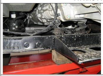
9. Using a jack support transmission cross member and remove mounting bolts. Fit rear mounting bracket using original bolts and tighten. Remove jack from vehicle.
