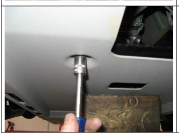
12. Secure rear of panel using 2 x M8 x 25 bolts, spring washers, flat washers and M8 flange nuts. Once all is fitted correctly tighten all bolts.
