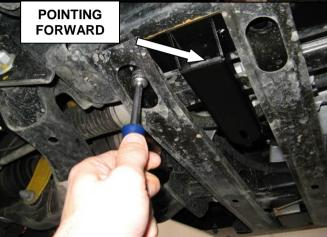
6. Slide middle mounting bracket over skid rail mounting points making sure mount tabs point forward. Re-fit and tighten original bolts as removed in step 2.
